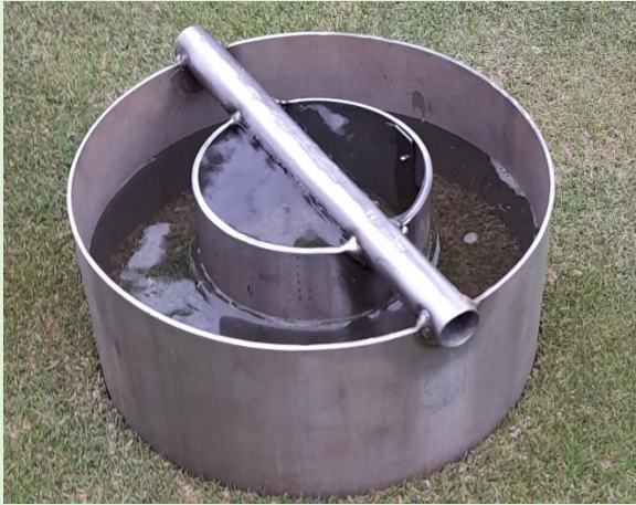
Measuring the ability of the surface to vertically percolate the water through the profile. (mm/hr).
