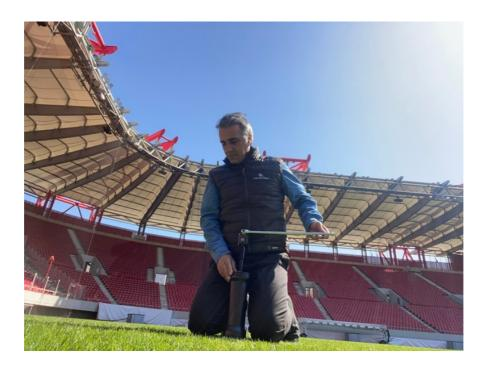
The ProPitch Light Weight Rotational Resistance apparatus simulating underfoot friction or grip a player may experience when changing direction or speed.
